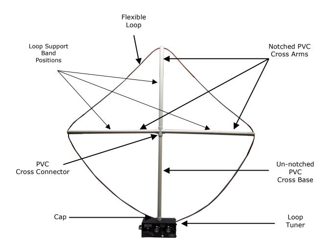
Figure 1: PVC Cross Mount Loop Assembly
